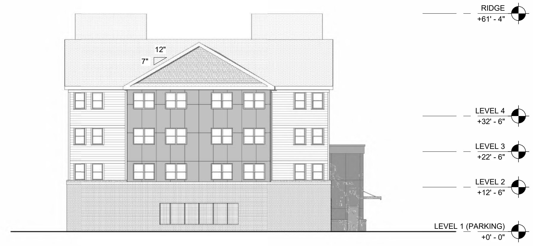
3 EXTERIOR ELEVATION - NORTH 1/16" = 1'-0"
