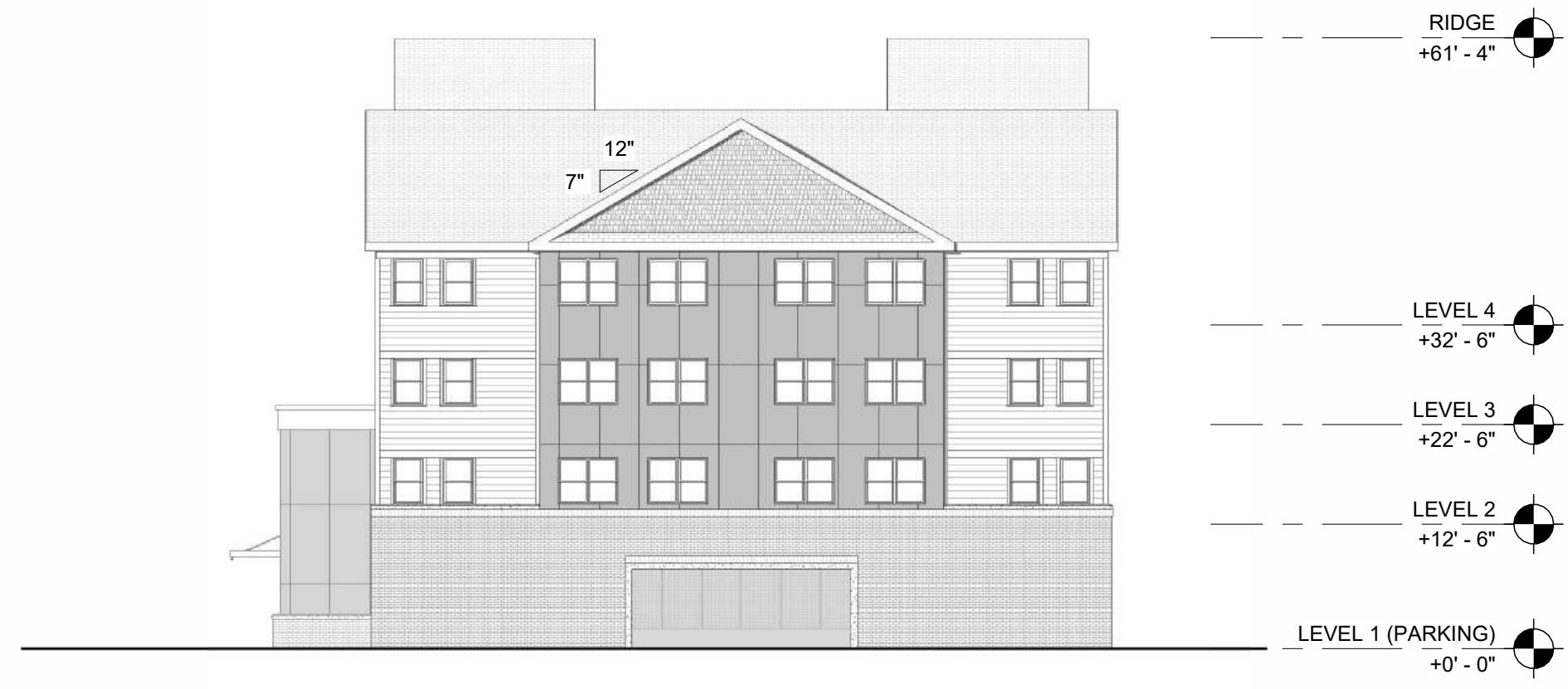
4 EXTERIOR ELEVATION - SOUTH 1/16" = 1'-0"
